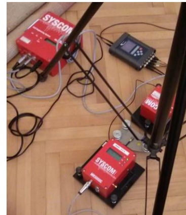
Figure 6. Vibration measuring system with triaxial acceleration sensor based in the center of the room below dummy head measurement system
