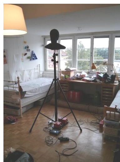
Figure 3 – Measuring Point 3, single house, 2 nd floor, dummy head
