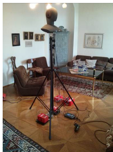
Figure 5 – Measuring Point 5, flat, 2 nd floor, dummy head
