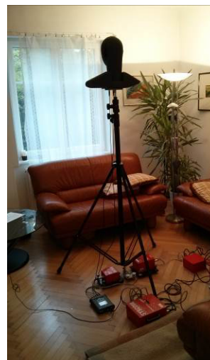
Figure 4 – Measuring Point 4, single house, ground floor, dummy head
