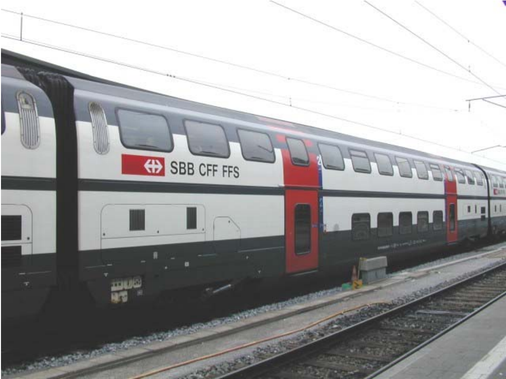
Well covered bogies of Swiss passenger wagon IC2000
